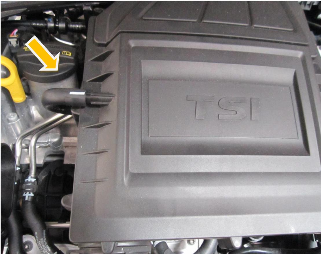
3. Using a T30 Torx Drive undo the fastener that holds the airbox in position.
