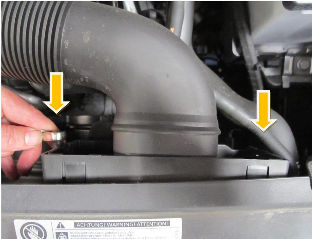
6. Pull the airbox sharply upwards to remove.
