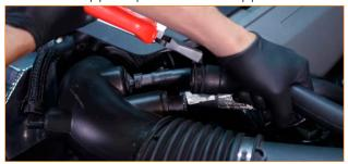
03. If you want to delete your sound generator, loosen the clamp at the other end of the sound-generator hose. Remove the hose by lifting it upward near the clip that secures the hose to the airbox. Follow the sound-generator tube back to the firewall and remove the nut that secures it. Then remove the sound-generator tube and install the provided firewall plug to seal the port. (1x 10mm nut, 1x spring-clamp, 1x worm-gear clamp)
