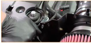
24. Locate the intake hose and remaining hardware in your kit. If you choose to retain your sound generator, you will install the barbed port. If you choose to delete the sound generator, you will install the Mishimoto branded plug. Secure the port or plug with the provided worm-gear clamp. (1x plug or port, 1x small worm-gear clamp)
