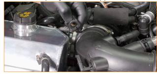
05. Remove the rear hose from the intake pipe using the same process.
