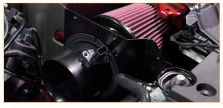
23. Lead the MAF wiring around the corner of the airbox and secure it with the integrated tree-clip.
