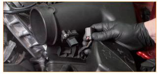
11. Remove the bolt that secures the airbox to the vehicle.
